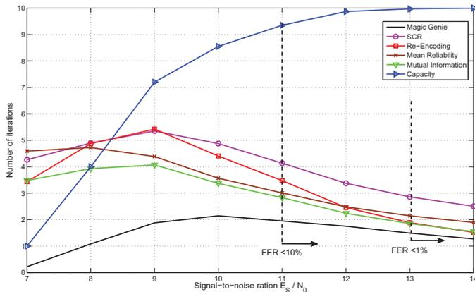
Fig. 6. Average number of iterations of different iteration control metrics versus signal-to-noise ratio
