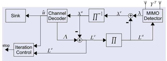
Fig. 3. Iterative MIMO-BICM receiver including iteration control based on channel decoder outputs
