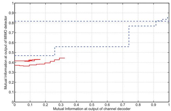
Fig. 2. EXIT chart showing the typical behavior of decodable (dashed lines) and non-decodable (solid lines) blocks during iterative detection and decoding of the analyzed MIMO-BICM system
