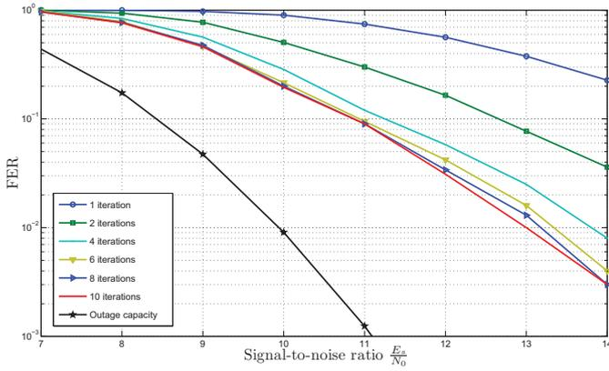
Fig. 4. Frame error rate versus signal-to-noise ratio for different number of iterations
