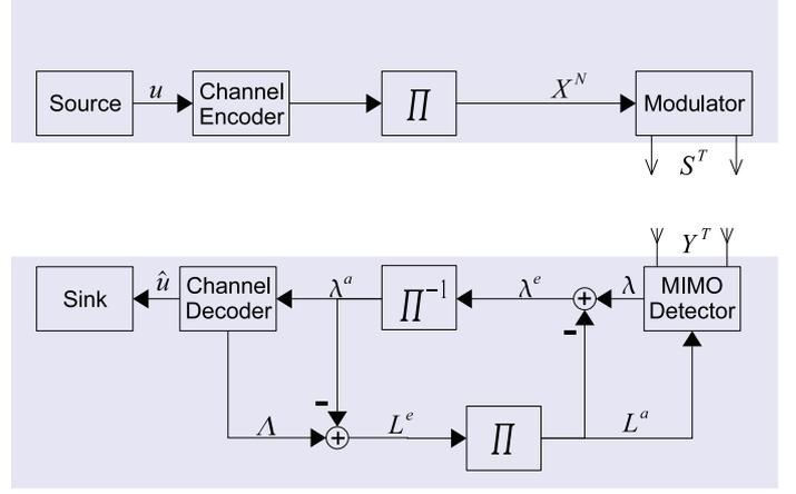
Fig. 1. MIMO bit interleaved coded modulation system model
