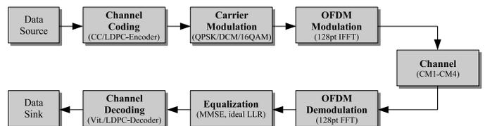
Fig. 1. WIMEDIA UWB simulation chain
