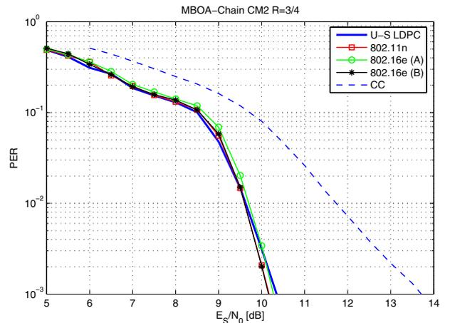
Fig. 7. Communications performance in the CM2 channel
