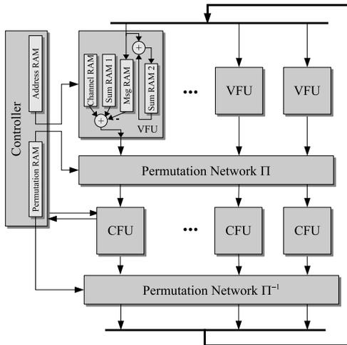
Fig. 4. Two-Phase Decoder Architecture
